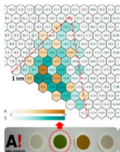
Figure 1. (n,m) distribution of the green SWNTs and photos of the SWNT thin films synthesized at 850 °C. with 0 %, 0.25 % (green), 0.37 % (brown) and 0.5 % of added CO 2 .
